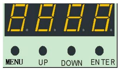
Menu key: Select functions Up key: parameter increments Down key: indicates the descending parameter value Enter key: Confirm and save
